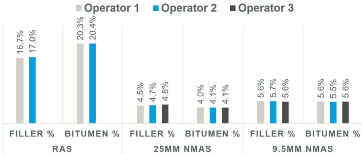
**Figure 3** The Impact of Operator Error on Asphalt Binder Content and Percentage of Fines
