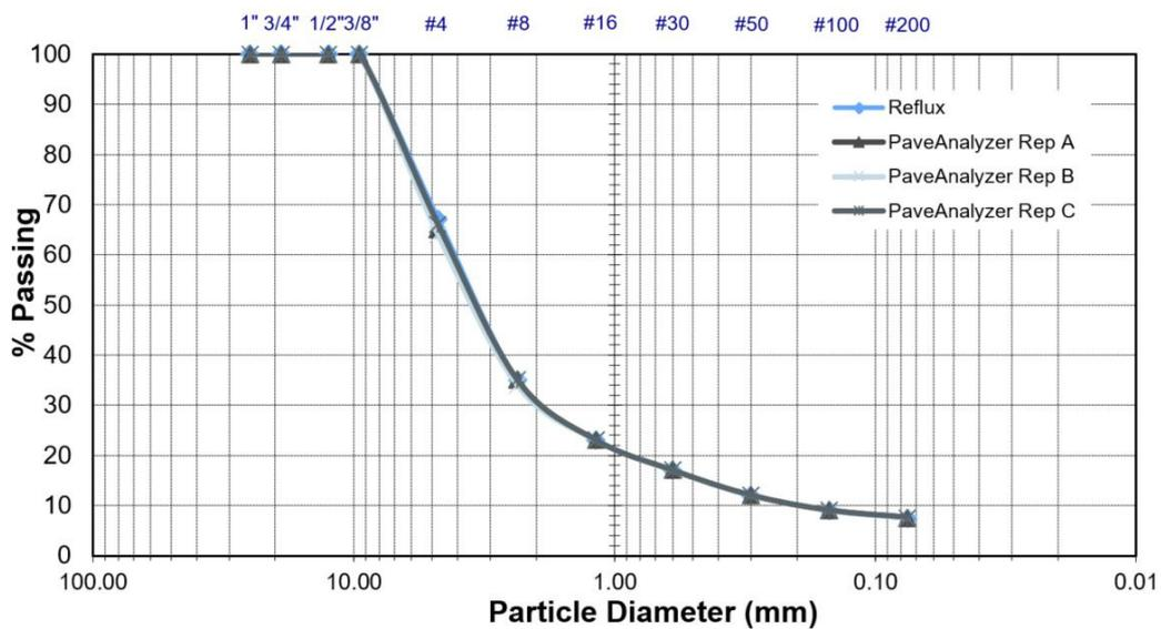
Figure 4 Comparison between Aggregate Gradations after Extraction Using Reflux and PaveAnalyzer
