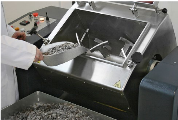
77-PV0077/C Detail of aggregate loading
