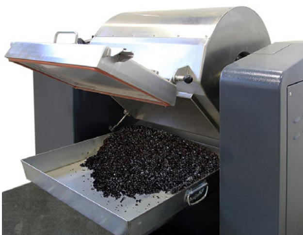
77-PV0077/C Detail of unloading. The mixing cylinder is rotated by a motorized tilting system for easy unloading. The tilting angle is adjustable to 130° to speed up the unloading operation.
