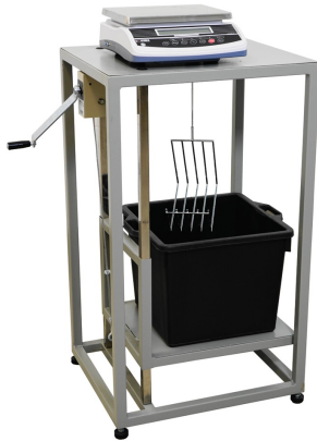
Specific gravity frame with electronic balance and cradle for specimens
