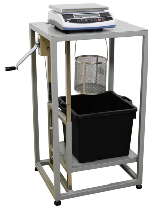
Specific gravity frame with electronic balance and basket
