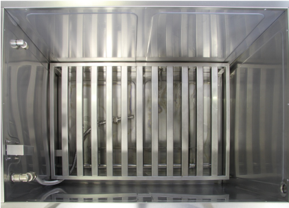
Programmable accelerated curing tank, detail of base supporting grid
