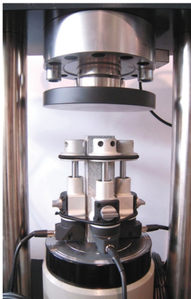
Three compressometer-extensometers 55-C0222/F fitted to a mortar prism 40x40x160 mm
