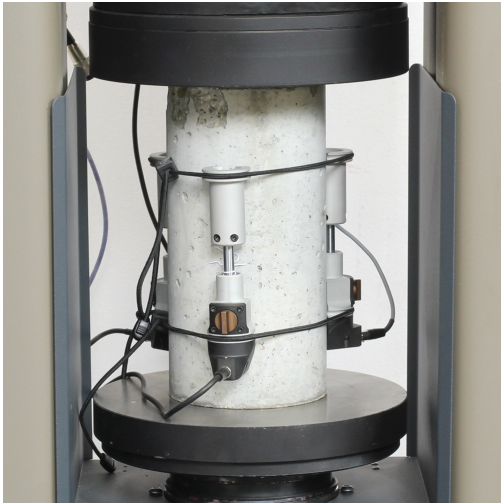
Three compressometer-extensometers 55-C0222/F fitted to a cylindrical specimen during compression stage.
