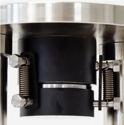
Compression device for rock specimens model 32-D9035: detail of the spherical seat hold by springs
