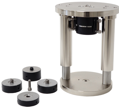
Compression device for rock specimens model 32-D9035: detail of the distance pieces included in the jig
