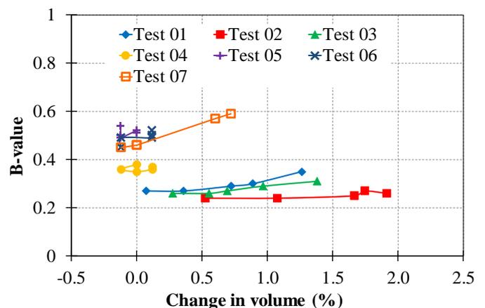
Figure 5 B-value versus volume change for Stage 1 in all seven tests (Back Pressure=50kPa)
