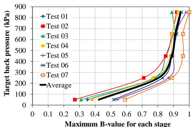
Figure 2. Plot of B-value versus target back pressure
