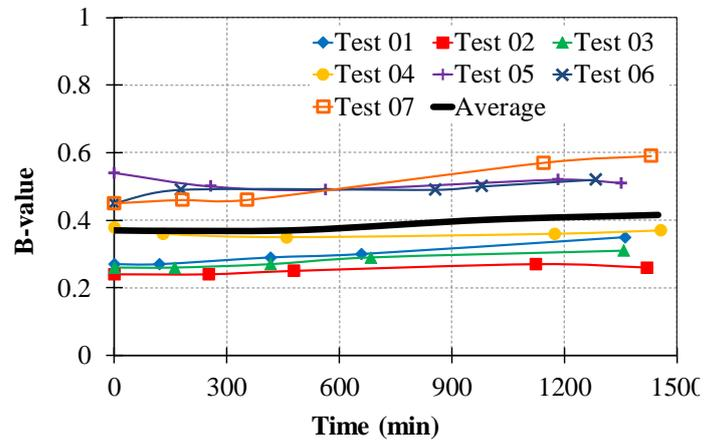
Figure 4. B-value versus time for Stage 1 in all seven tests (Back Pressure=50kPa)
