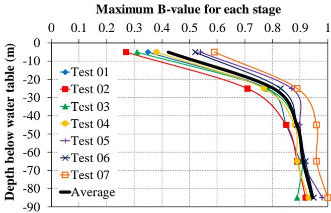
Figure 3. Plot of B-value versus depth below water table
