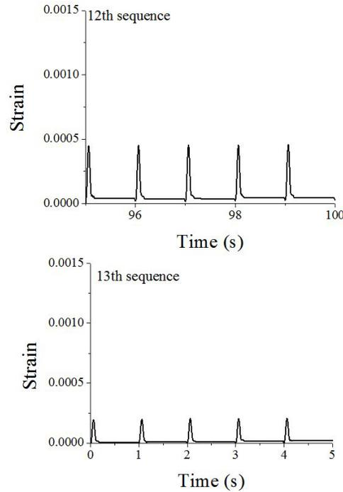
Figure 3b. Strain response during 12th and 13th sequence for BSM
