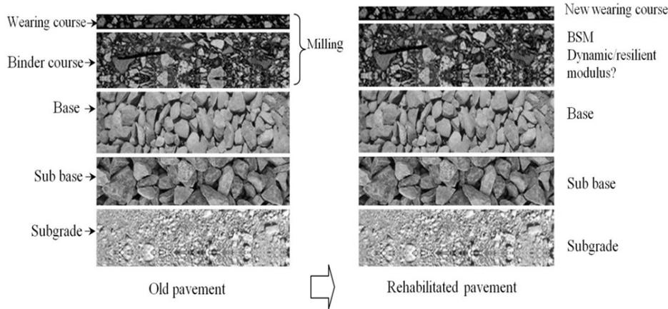
Figure 1. Cross section of a pavement ( M-E PDG, 2004)
