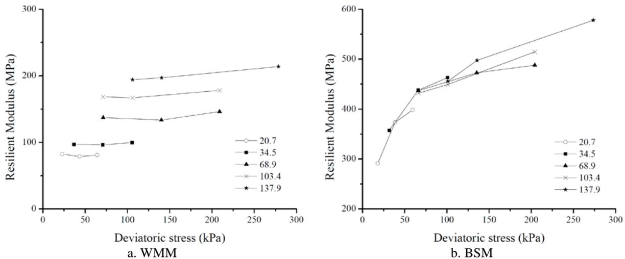
Figure 5: Resilient modulus as a function of deviator stress at various confinement pressure
