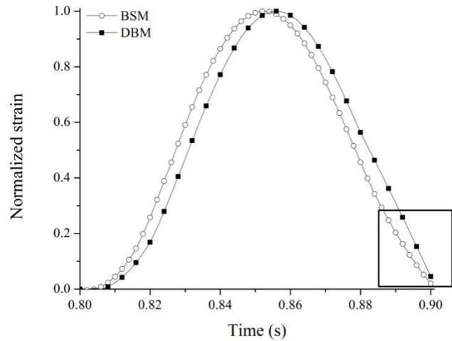
Figure 8b. Normalized strain during dynamic modulus test
