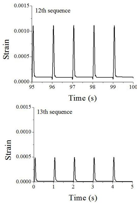
Figure 3a. Strain response during 12th and 13th sequence for WMM
