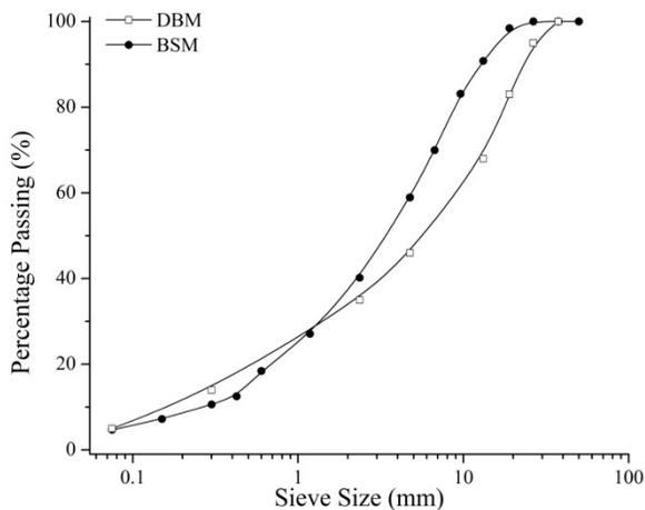
Figure 6. Gradation of BSM and DBM
