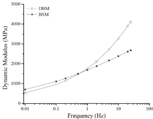
Figure 7a. Dynamic modulus as function of frequency
