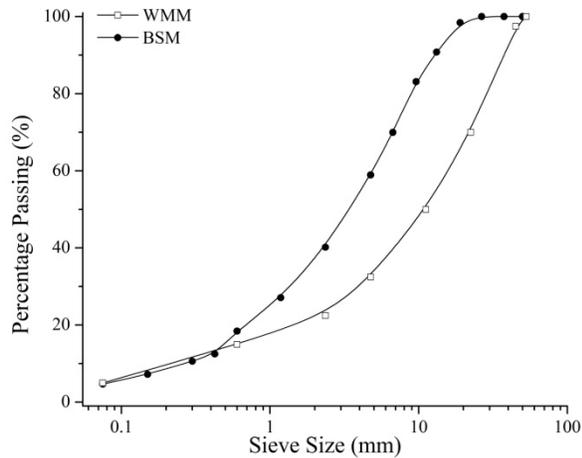
Figure 2. Gradation of BSM and WMM
