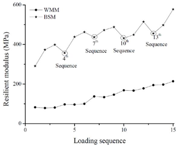
Figure 4. Resilient modulus for the entire 15 loading sequences
