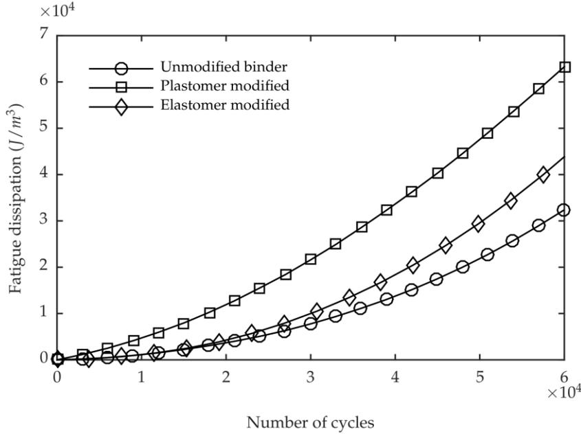
Figure 3. Variation of cumulative fatigue dissipation with the number of cycles of repetition for the bituminous mixtures
