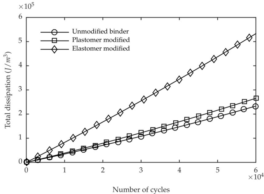
Figure 2. Variation of cumulative total dissipation with the number of cycles of repetition for the bituminous mixtures
