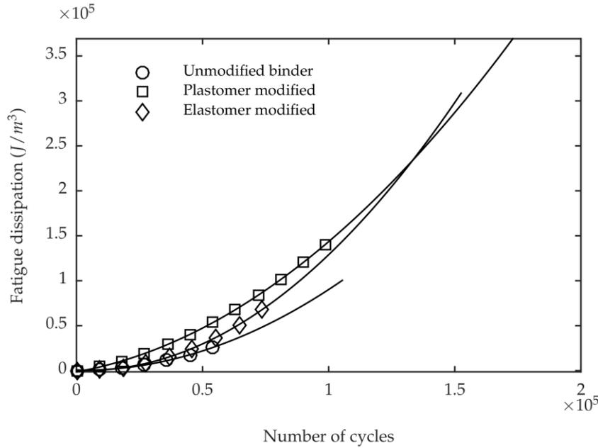
Figure 4. Quadratic polynomial fit to the cumulative fatigue dissipation curves and extended up to the point of failure
