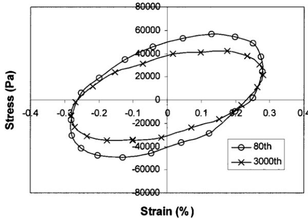
Figure 1. A sample displacement-controlled fatigue test result with total dissipation in a cycle decreasing with each cycle (Source: Kim et. al. (2003))
