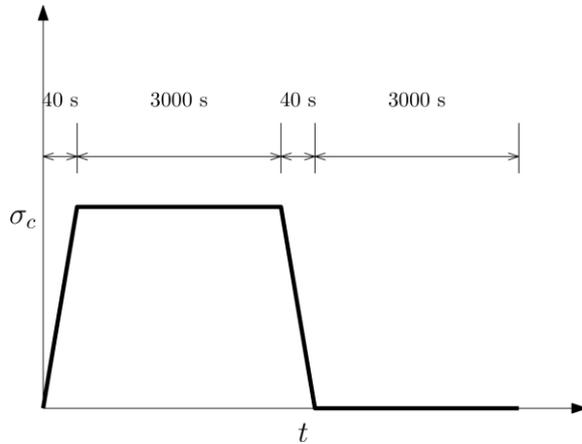
Figure 3. Schematic representation of the confinement pressure creep-recovery test
