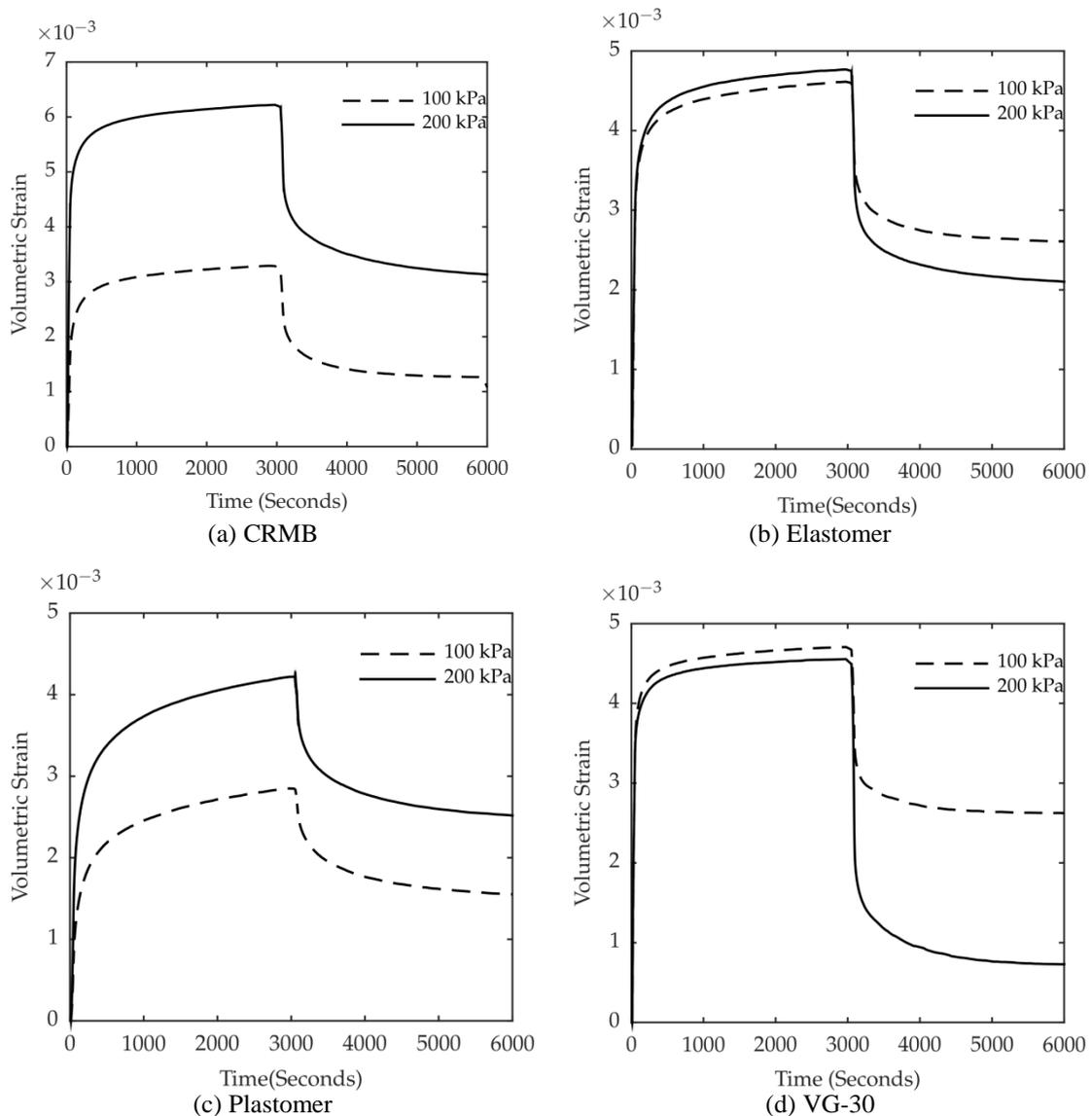
Figure 5. Comparison of volumetric strain of different binders at 100 kPa and 200 kPa pressure
