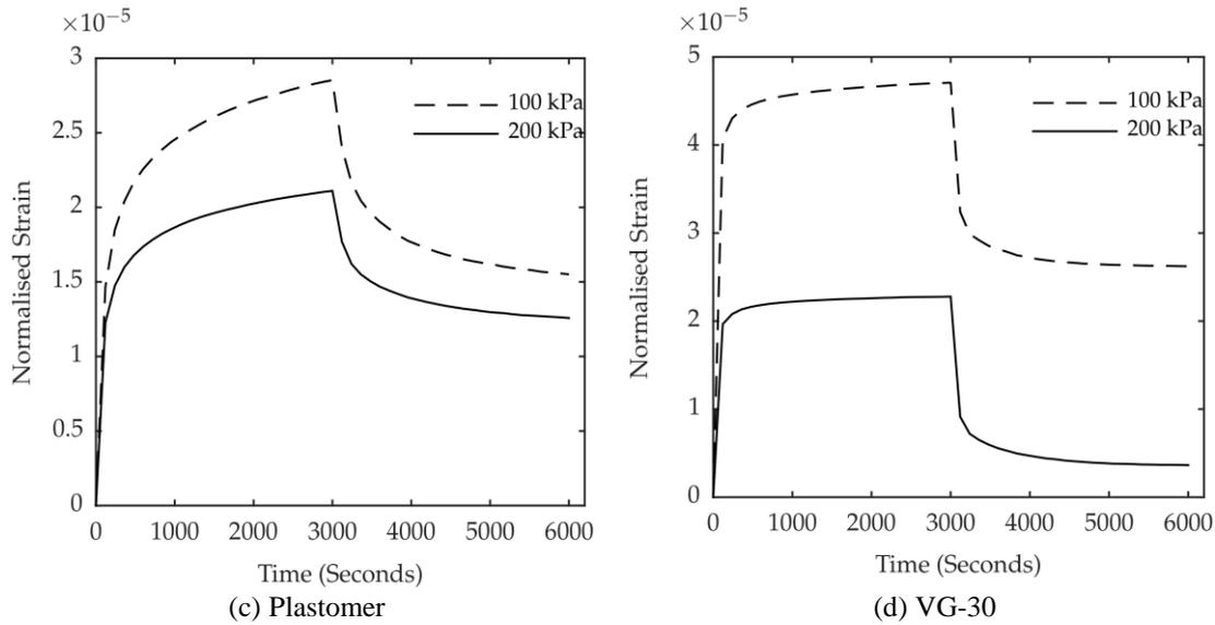
Figure 6. Check for linearity of creep-recovery response
