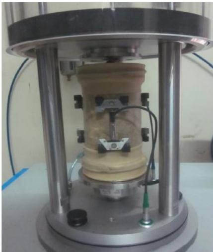
Figure 2. Experimental set up for pure confinement creep and recovery experiment
