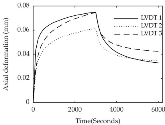
Figure 4. Axial strain history of bituminous mixture with plastomer at 100 kPa pressure
