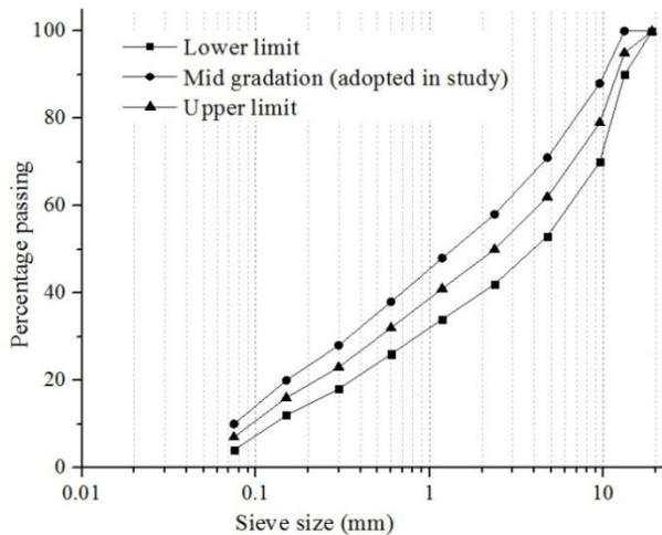
Figure 1. Gradation of the mix used for the study
