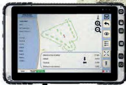
**Wirtgen's AutoPilot 2.0 can test slipforming data for kinks and display them on the system's tablet**
