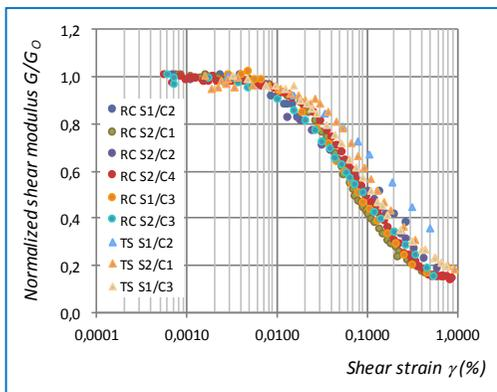
Figure 2 Reduction curves of Shear Modulus
