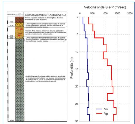
**Figure 1 Profiles of the velocities obtained from a DH test.**
