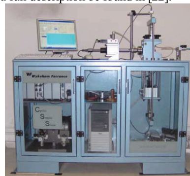
Figure 2. Cyclic DSS equipment used for the tests.
