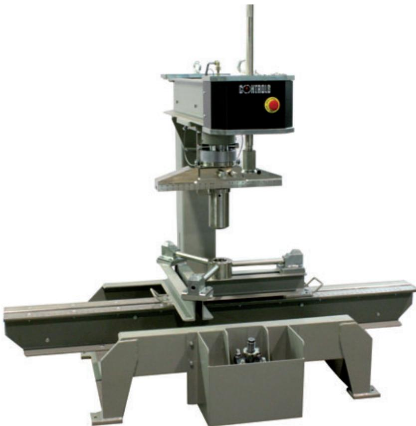
Fig. 1: Model 50-C1601/FR 300kN high stiffness frame, the test configuration conforming to ASTM C1550
