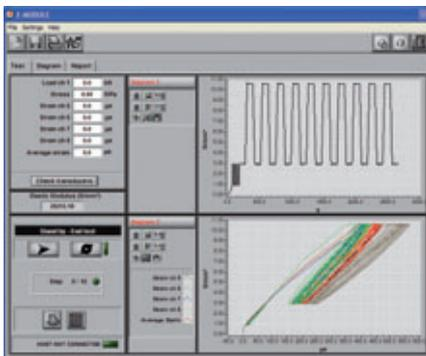
Fig. 3: Main window of the E-Module software for the automatic determination of the Elastic Modulus.
