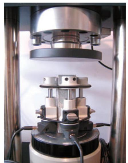
Fig. 1: Concrete and mortar specimens fitted with high precision 55-C0222/F sensors for EM test
