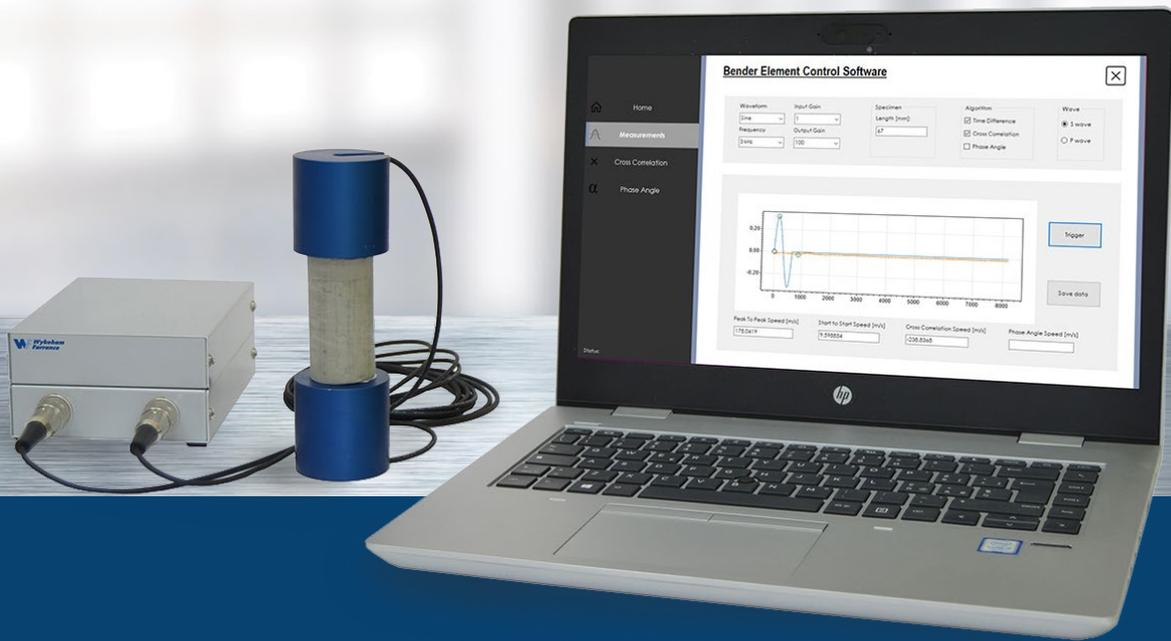
Bender elements allow you to measure the maximum shear modulus ( $G_{max}$ ) of a soil sample in order to evaluate its stiffness.  $G_{max}$  — typically with shear strain levels of about 0.001% — is a key parameter in low-strain dynamic analysis used to predict soil behaviour or soil structure interaction during earthquakes, explosion or machine and traffic vibrations.
