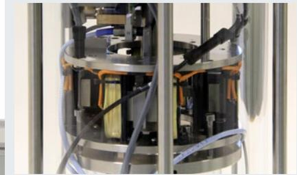
**Internal floating frame** for assembling the electrical motor that applies torsional loads.
