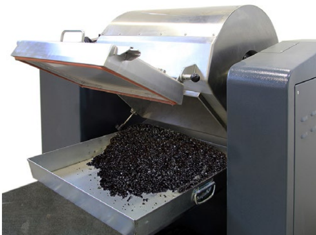
77-PV0077/C Detail of unloading. The mixing cylinder is rotated by a motorized tilting system for easy unloading. The tilting angle is adjustable to 130° to speed up the unloading operation.
