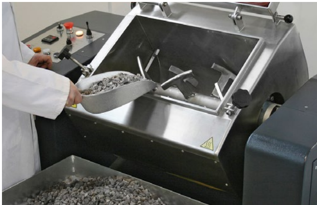
77-PV0077/C Detail of aggregate loading
