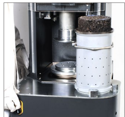
Integrated worktop with electromechanical extruder option 78-PV2520/15
