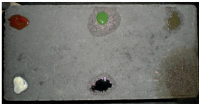
Fig. 6: MasterPel 500 (100 g/m<sup>2</sup>) – application of the staining agents on wet surface
