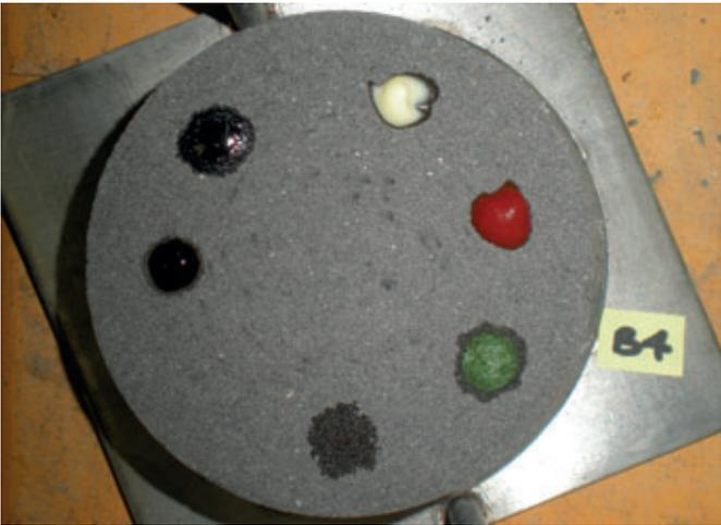
Fig. 1: Reference – application of the staining agents on dry surface
