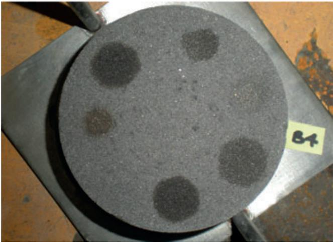
Fig. 2: MasterPel 500 (100 g/m<sup>2</sup>) – application of the staining agents on dry surface
