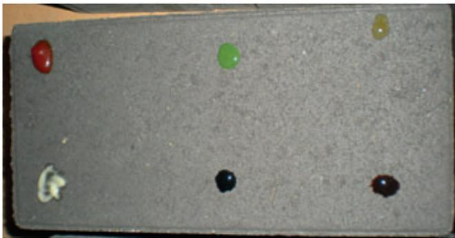
Fig. 8: MasterPel 500 (100 g/m<sup>2</sup>) – after treatment with 5% HCl solution
