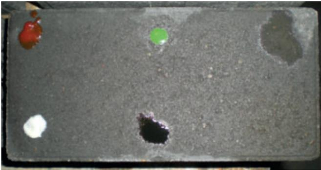
Fig. 5: Reference – application of the staining agents on wet surface
