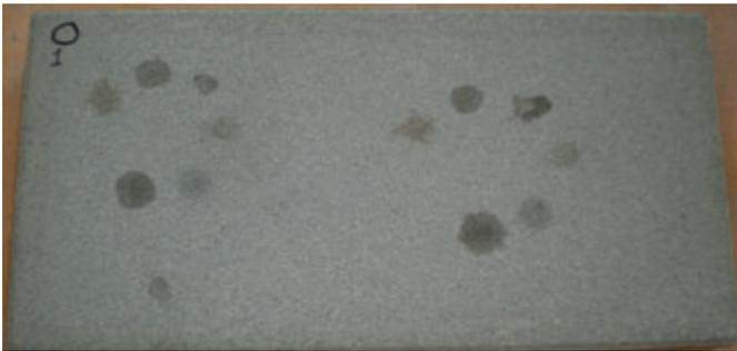
Fig. 4: MasterPel 500 (100 g/m<sup>2</sup>) – application of the staining agents on dry surface
