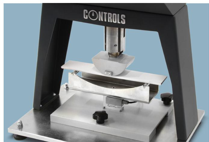
Detail of load cell, test supports and loading anvil
