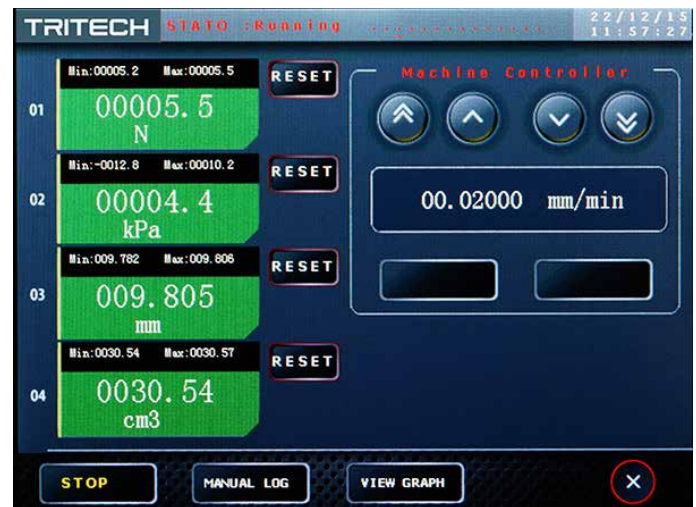
Transducer live display screen during the test
