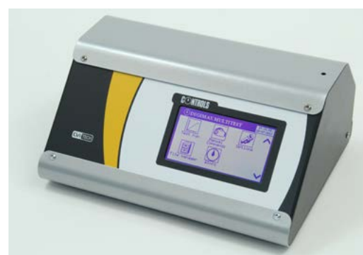
Digimax data acquisition and processing unit (included with Marshall tester 76-B3802)
