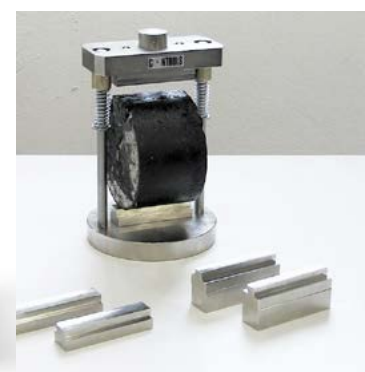
Tensile splitting device (Lottman breaking head) 76-B0078/C with strips 76-B0078/C1 and C2
