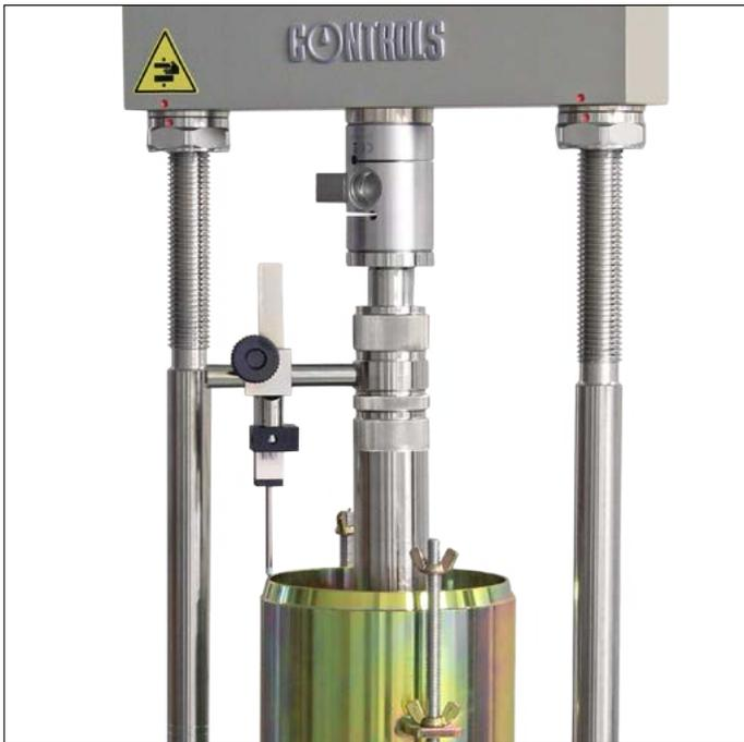
*Detail of the accessories to perform the CBR test in the digital mode*
