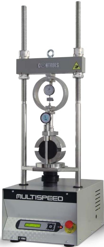
Universal compression tester Multispeed 34-V1072 with Marshall accessories in the analogical mode
