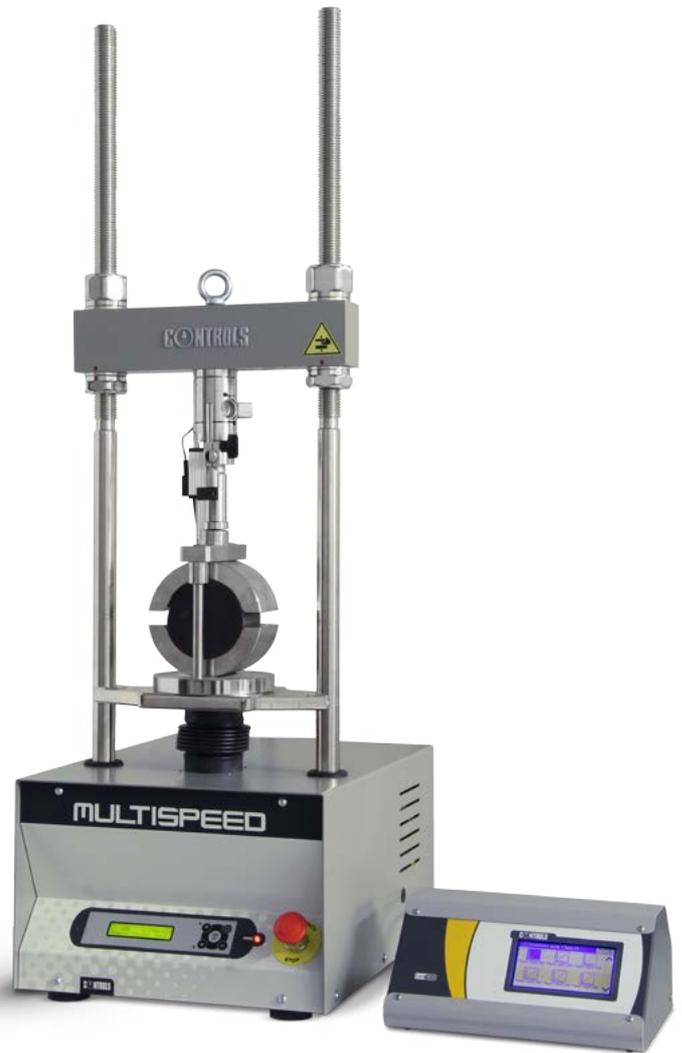
Multispeed 34-V1072 fitted in the digital mode to perform the Marshall test, complete with the Digimax TS unit
