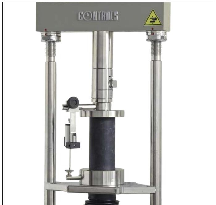
*Detail of the accessories to perform the Unconfined test on soil in the digital mode*
