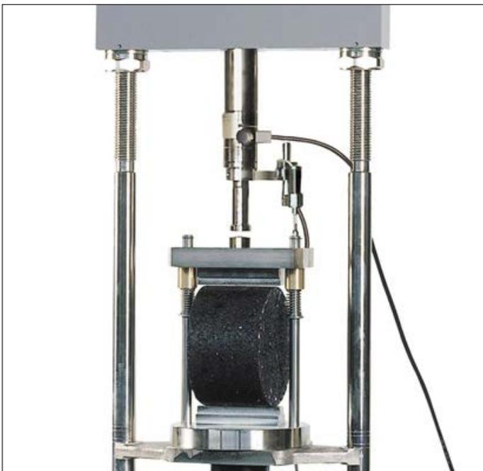
*Detail of the accessories to perform the indirect tensile test in the digital mode*
