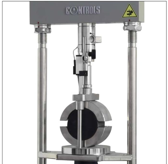
*Detail of the accessories to perform the Marshall test in the digital mode*
