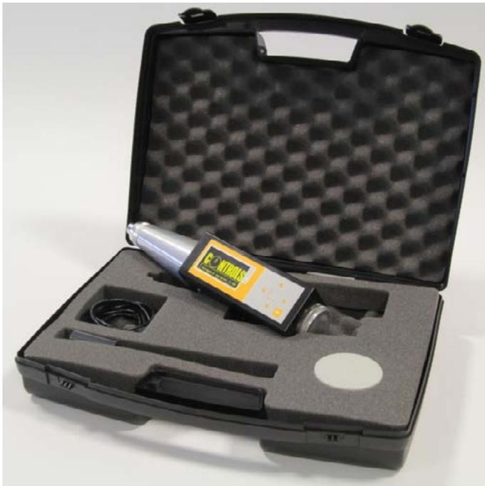
Rebound digital test hammer supplied complete with case (model 58-C0181/DGT)
