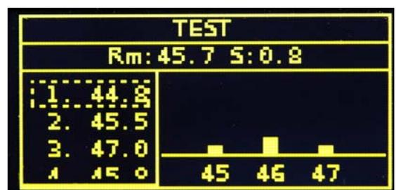
Example of digital hammer screen display - Test results displayed as numerical and graphical format
