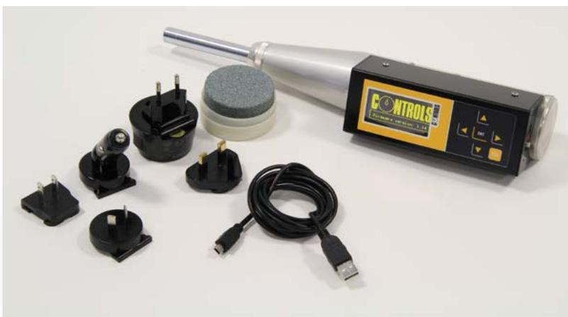
Rebound test hammer digital model 58-C0181/DGT
