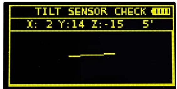
Example of digital hammer screen display - Measurement and indication of the exact instrument tilting angle by triaxial inclinometer
