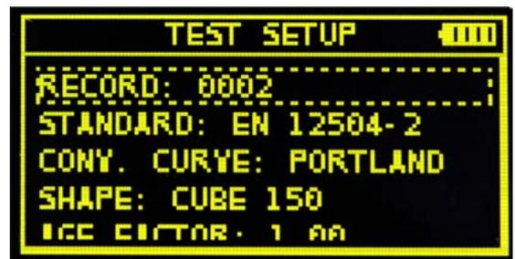
Example of digital hammer screen display - Test setup
