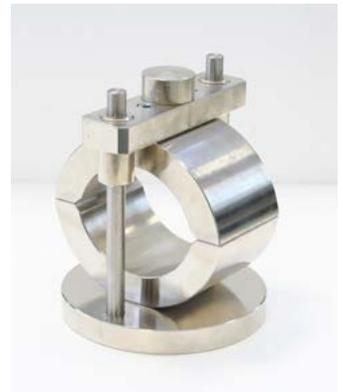
Marshall stability mould for 4" dia. specimens 76-B0033
