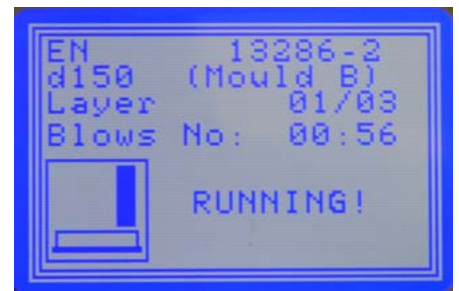
Compaction progress view
