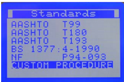
Compaction test procedure selection (display)
