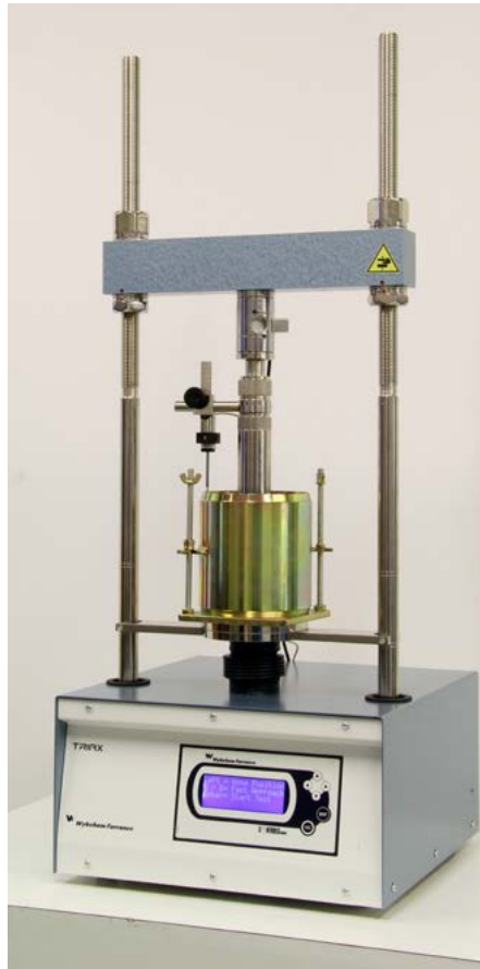
Load frame 28-WF4001 with CBR digital configuration
