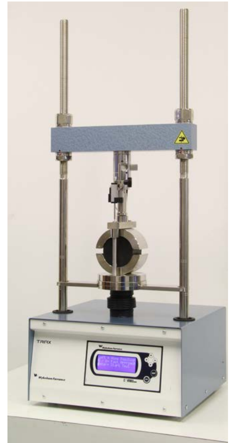
Load frame 28-WF4001 with Marshall digital configuration
