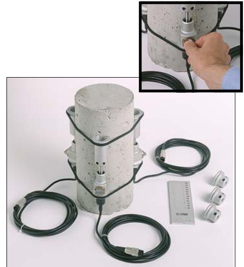
Dia 150 x 300 mm cylinder fitted with 3 55-C0222/F ready for an elastic modulus test. The detail above shows the lock/unlocking device of the transducer.
