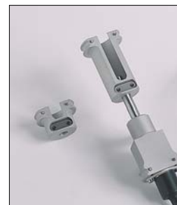
Contact face of the instrument. Note the 4 hardened steel points which prevent slippage.
