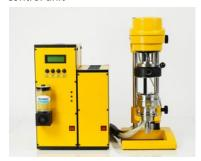
Peltier unit: Peltier control unit, peltier temperated basic plate, basic plate support, adapter, exchange grip, exchangeable plate (ø 25mm), measuring plate P3 (ø 25mm), measuring plate P4 (ø 8mm)
