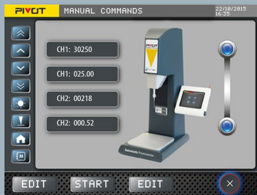
Alternative manual adjustment of the needle position
