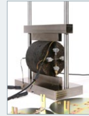
AASHTO T322/TP9, ASTM D7369, & NCHRP 1-28A APPENDIX 1
