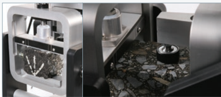
Four Point Bend Jig
