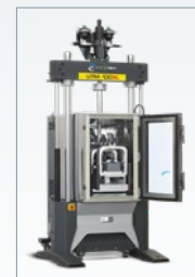
Extra Large Four Point Bend Jig inside UTM-130XL
