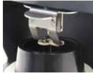
Detail of the new needle cleaning device. Functionality is substantially improved respect older versions following suggestions received from end-users
