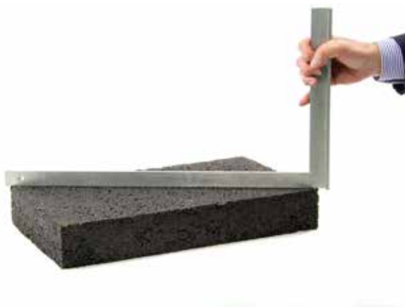
Planarity, Regularity and homogeneity of the slabs produced by the roller compactor
