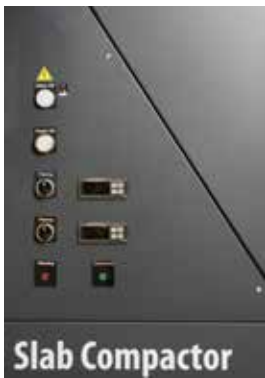
Detail of the control panel for controlling the temperature of sector head and base heating system
