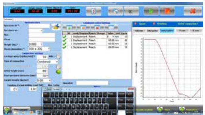
Combined load/displacement Compaction
