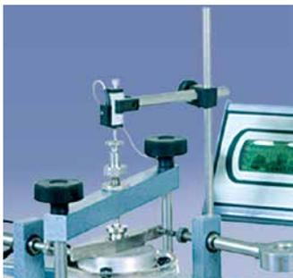
30-WF6207 Linear potentiometric transducer
