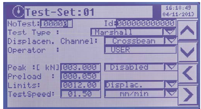
Marshall data display during test with 70-V1172 MULTISPEED universal tester
