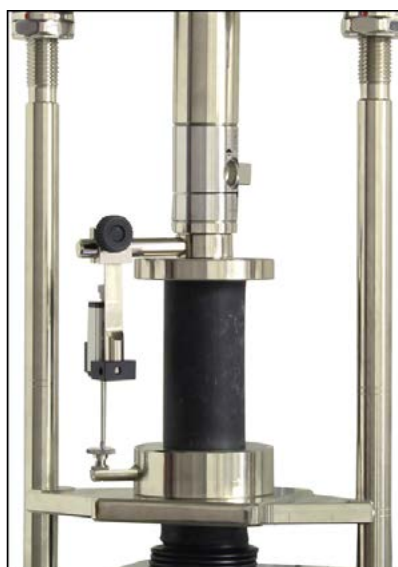
Unconfined compression accessories assembled on Universal compression machine 70-V1172
